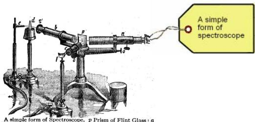
A simple form of Spectroscope. p Prism of Flint Glass; a Telescope with Eyepiece; b Collimator through which the Light, which enters at the Slit in the End s from the Flame of the Bunsen Burner d, passes to the Prism to form Spectrum in a; c Tube with a Micrometer; e Holder for Substance whose Spectrum is to be examined; f Flame illuminating Micrometer Scale; o o Adjusting Screws.
